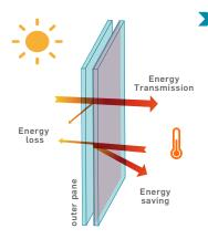
Neutralux® technology enables control of the transfer of heat energy to the outside and provides low emission properties.
